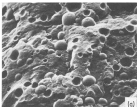
Figure 2 Scanning electron micrographs of cryogenic fracture surfaces of B blend extruded at 220°C with different residence times: (a) 3 min, \times 3750 ; (b) 10 min, \times 3750 .
